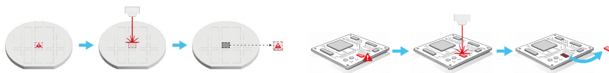
Left: selective defect removal on a wafer. Right: selective defect removal on a board. Both applications enabled by microPREP®L. Copyright: 3D-Micromac AG.
