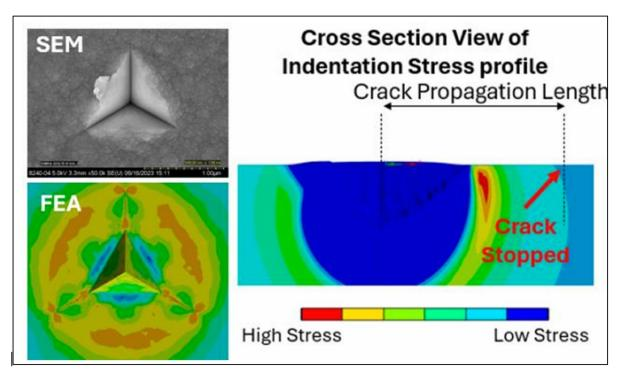
• The image above compares (on the left side) an SEM view of a deliberately induced crack in an SiO<sub>2</sub> thin film with the FEA prediction of what it would look like, showing excellent agreement. The right side of the image is an analysis of the calculated "stress intensity factor," which corresponds to the actual crack propagation length.
