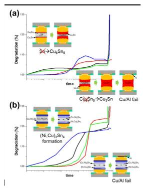
• <u>The image above</u> is a schematic diagram showing how the microstructures of (a) Cu/Sn and (b) Cu/Ni/Cu/Sn <u>non-full IMC</u> microbumps changed during electromigration testing, culminating in the failure of aluminum traces.
