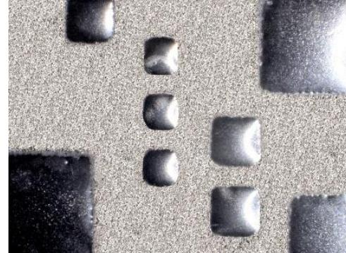
[MICRONOX MX2123](#) is a balanced, multi-phase chemistry designed to remove flux residues from a wide range of IGBT module devices that utilize combinations of copper, silver and nickel DBC as substrates. It can also remove fluxes from PCBs. MX2123 can remove slight metal oxidation from base metals for post wire bond and potting processes, leaving exceptional surface conditions after cleaning.
