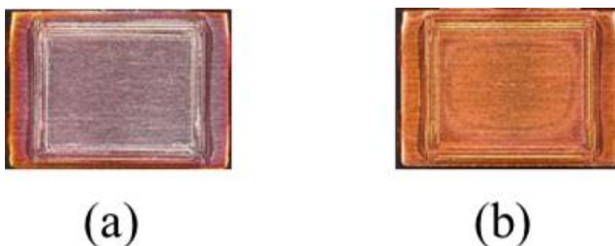
Fig. 5: Appearances of baked (a) non-coated and (b) coated Cu lead frame.
