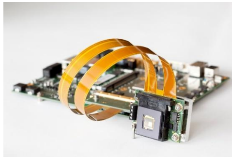
Customer Evaluation Kit with control electronics, connection cable, and 256 x 256 mirror device © Fraunhofer IPMS
