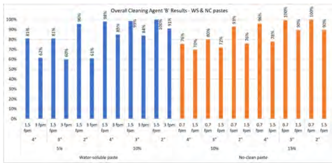
Figure 28. Cleaning Agent 'B': Overall cleanliness rating for both WS and NC pastes
