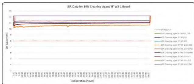
Figure 56. IPC-B-52 Vehicle – 10% Cleaning Agent ‘B’ WS-1 – Passed
