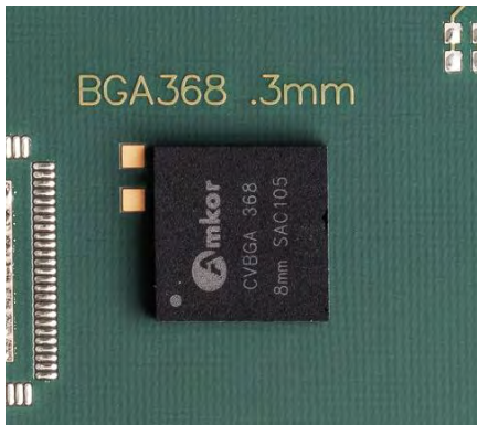
Figure 11. BGA368 Component Before Cleaning
