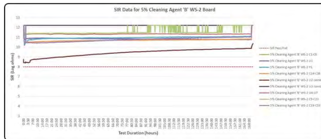
Figure 54. IPC-B-52 Vehicle – 5% Cleaning Agent ‘B’ WS-2 – Passed
