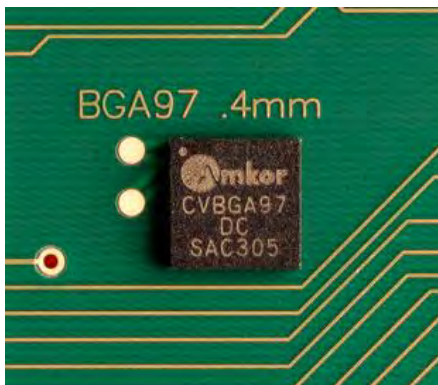
Figure 12. BGA97 Component Before Cleaning
