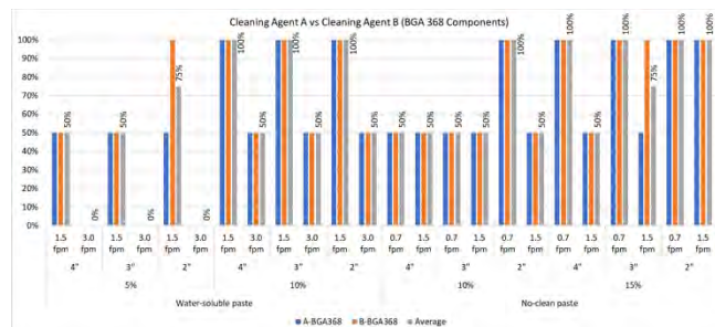
Figure 37. Cleaning Agent 'A' vs Cleaning Agent 'B': Cleanliness rating under BGA 368 components
