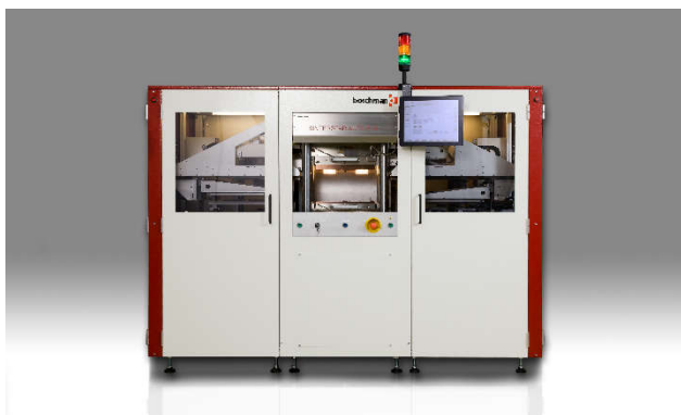
Fully automatic Ag- Sinter system: Sinterstar Inline-F-XL-HC
