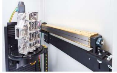
tested with the same X-ray energy. The solid housing is particularly resistant to temperature fluctuations, ensuring optimized cooling of the electronics. At the same time, it ensures very little scatter within the detector, resulting in much sharper images, cleaner edges and an improved detail detectability.
