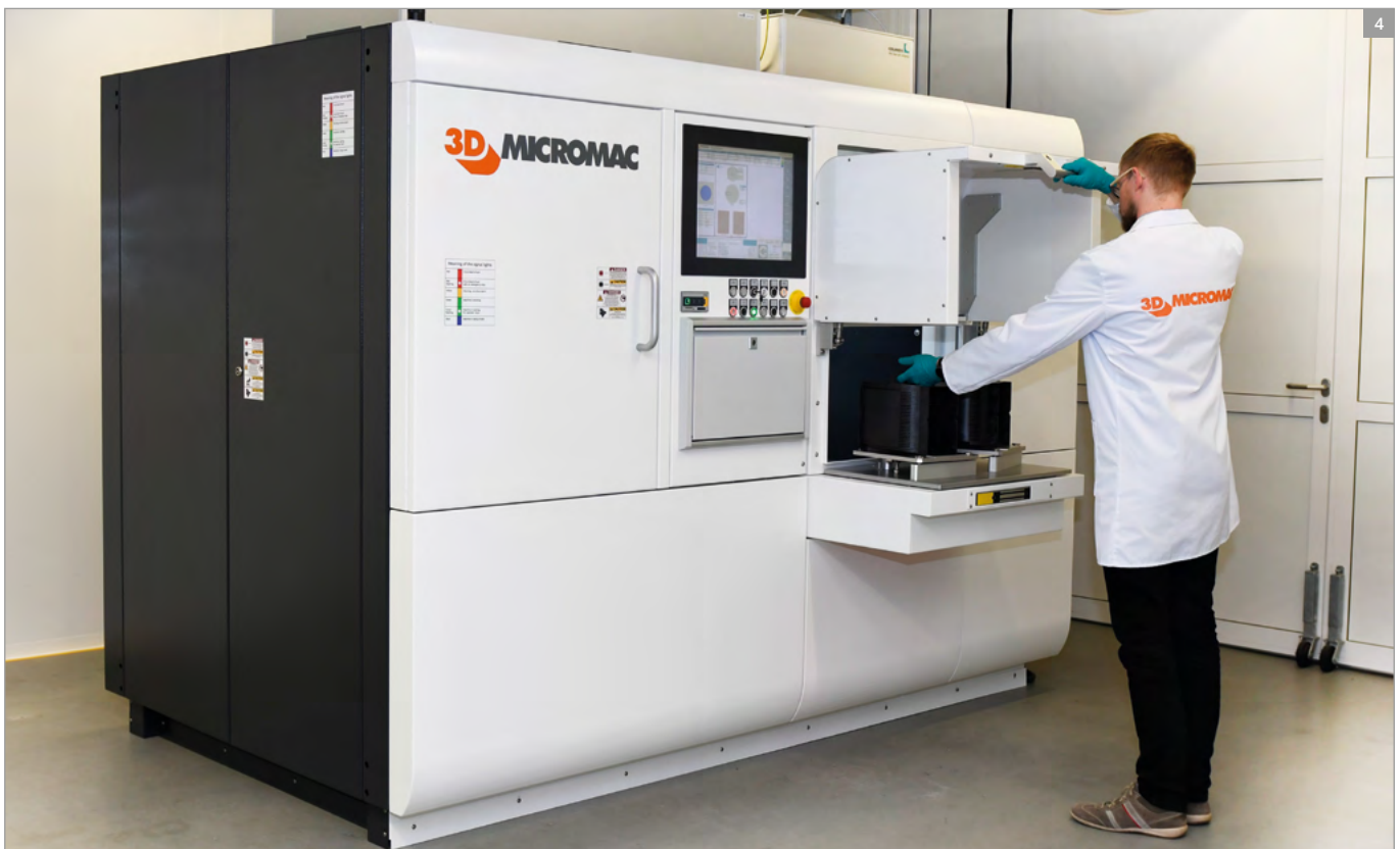
Fig. 4: microVEGA xMR selective laser annealing system for monolithic magnetic sensor formation.
