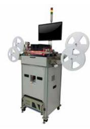
TR2000i offers three-in-one inspection, including leaded package inspection, ball package inspection and leadless package inspection, which can reduce maintenance costs, as well as mark and package inspection. TR2000i is able to inspect various types of 2D and 3D defects for various package sizes with high-speed, high accuracy and low false call.
