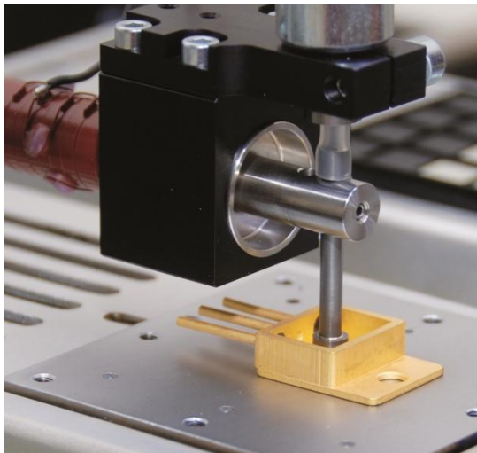
Figure 3: U/S process setup in a TRESKY Die Bonder machine
