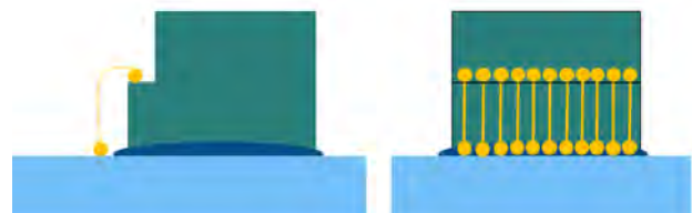
Figure 21: General layout of the assembly and wire bonds in this case study.
