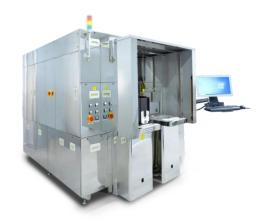
organic residues, and enabling flip chip packages to be manufactured at pitch dimensions down to 10 microns. The hydrogen plasma can also be used to remove fluorine contamination after plasma dicing on tape (PDOT). The plasma does not substantially heat the wafer and is safe for processing dies on tape frame.
