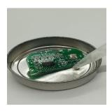
$e^{poxy}S^{et}$  supplies the SILCAST<sup>TM</sup> SC-417, optically clear, soft silicone for potting, sealing and encapsulating applications. This 1:1 mix system will cure overnight at room temperature or within 30 minutes at 150°C with a work time of about 30 minutes. The extremely low viscosity allows for penetration of components to yield a complete, air free potting.
