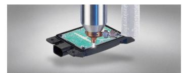
Surface pretreatment with plasma has significant effects on various processes, e.g. sealing in electronics. Thanks to Openair-Plasma and modern, solvent-free adhesives, these manufacturing processes are possible completely without wet-chemical waste.
