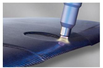
Openair-Plasma can be used in the automotive industry to optimize pretreatment processes, e.g. before painting, so that no VOC emissions are generated.
