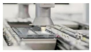
In the Semiconductor PTU, Openair-Plasma is used to effectively remove all organic and silicone-based contaminants as well as electrostatically charged dust. (Copyright: Plasmatreat GmbH)
