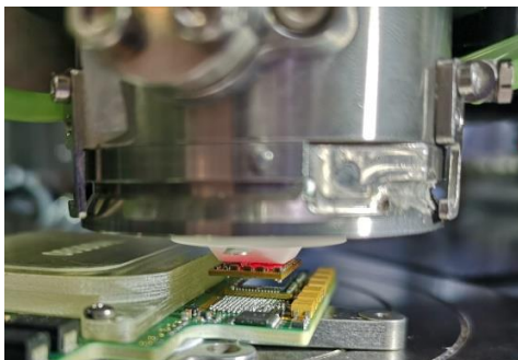
Fig. B2: Removal of a faulty PoP via LAPLACE LAdB
