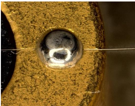
Fig. C3: SB 2 -WB wire bond on a sensor housing
