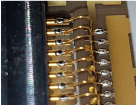
Fig. C2: SB 2 -WB wire bonds in a plug module
