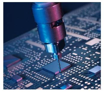
Henkel's portfolio of die attach solutions and underfill materials enables package design innovations for semiconductors.
