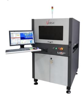
In addition MVPs platforms uniquely allow for multiple lighting options. If you need 3D imaging you can use the Versa Pro's multiple angled projectors and lighting options. If you need surface inspection you have the ability to use our advanced lighting solutions to enhance inspection and find many defects that would otherwise be hidden to other technologies.
