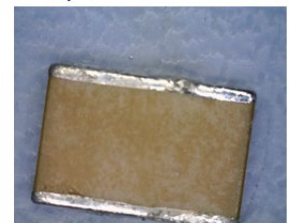
Board 2, C1 No Flux on cap underside, no visual residue on PCB
