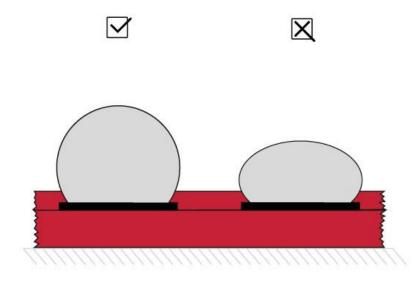
Low bumps are harder to grip. Therefore, the ball height-to-diameter ratio (diameter/height) should be less than 2,2. Solder balls with values above 2,2 should use shear testing. As always, the rule is to choose the test that gives the most failure modes of interest, and if none of them do this, select the test that produces the highest test forces.
