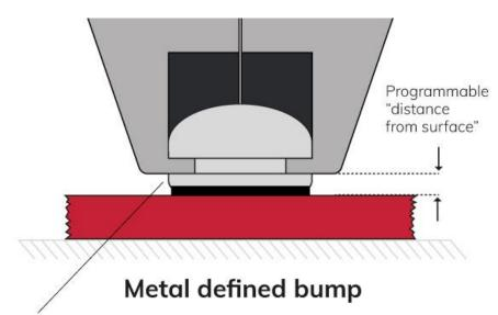
"Pull height" reduces stresses here on the bond caused when the ball is reformed
