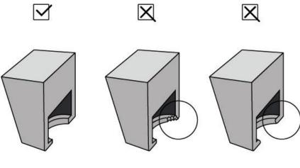
Good cavity Broken cavity Worn or round edge
