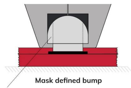
Reform the ball as low as possible to provide a maximum amount of solder above the grip edges for the maximum pull force possible
