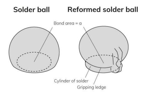
Ideally, the "stem" of the mushroom shape should be larger or the same diameter as the bond area. It is better if over gripping tests the bond at a higher force. Over gripping can still lead to getting a ductile break or extrusion, but the bond has been tested to the highest force possible.
