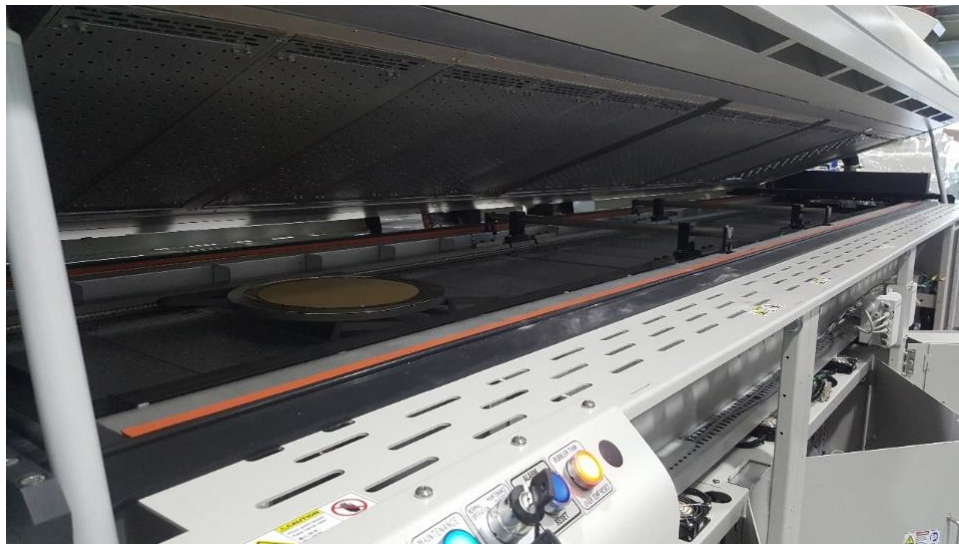
Exhibit 3: Wafer and Chuck Moving Through Reflow Oven
