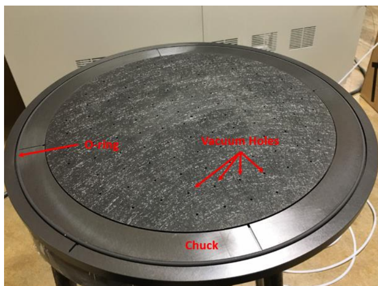
Exhibit 1: Wafer Vacuum Chuck for Film-Frame Wafer
