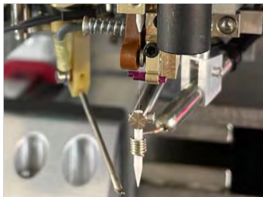
Figure 22: Thermally sensitive components can be wedge or ball bonded.
