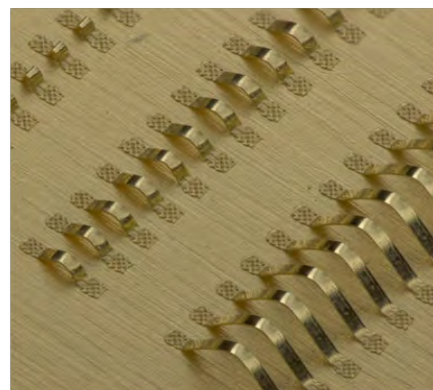
Figure 7: Typical ribbon bonding.
