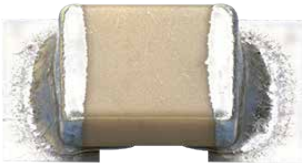
Figure 2 Shiny Solder Wetting
