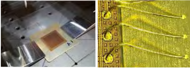
Figure 6: Test chip configuration with Au-wire-bonds on “F&S Bondtec system”. Left image shows the bond situation. Right image shows the TS-bonds.
