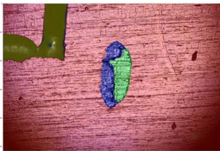
FIGURE 22: Image graded by trained U-Net 2 . Red: Background, Green: Ductile, Blue: Brittle, Yellow: Debris.
