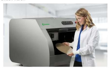
The standard configuration of W Series instruments includes 7.5 µm optics with molybdenum anode tube (chromium and tungsten are optional) and a high-resolution, large-window Silicon Drift Detector which processes more than 2 million counts per second. Silicon Drift Detectors are the standard, industry-wide, for complex films. Their high count rate capability is key to achieving a low minimum detection limit (MDL) and highest spectral resolution.
