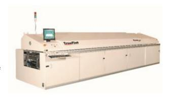
convection heating system. By eliminating die tilt and accommodating substrate thicknesses ranging from 0.15-0.30 mm, TrueFlat technology maximizes process yield.
