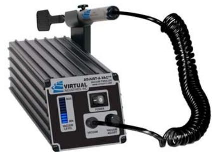
An integrated ten segment bar-graph-display visibly shows the vacuum level present during handling operations. Like the TWEEZER-VAC Elite, the system features an integrated bar-graph display and replaceable inlet filter that protects operation of the tool from dust particles. The TWEEZER-VAC Elite is available in various kits depending on your handling application. Kits are available in 110 or 220 volt operation.
