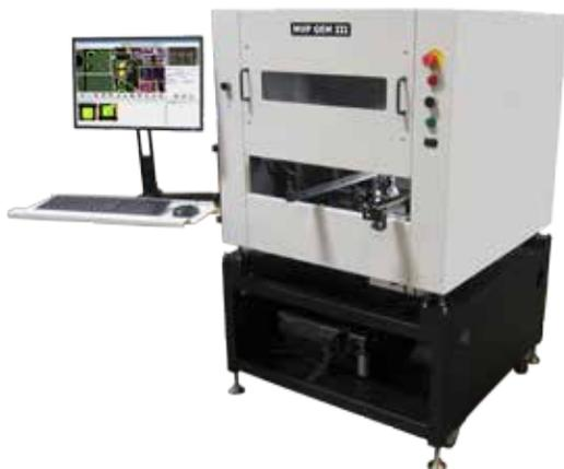
The GEM III AOI is a feature rich, highly robust, yet portable AOI platform based on Machine Vision Product's existing high performance AOI solutions. The GEM III incorporates an 8MP camera and is fully certified for 01005 inspection with an 8 micron pixel size.
