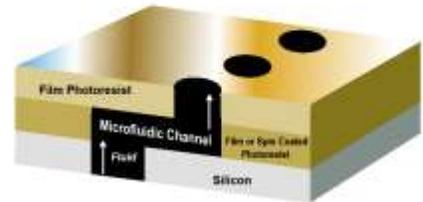
The 5  $\mu\text{m}$  dry film negative photoresist is the latest addition to Engineered Materials Systems' full line of film and liquid negative photoresists formulated for making microfluidic channels on MEMS devices and integrated circuits.
